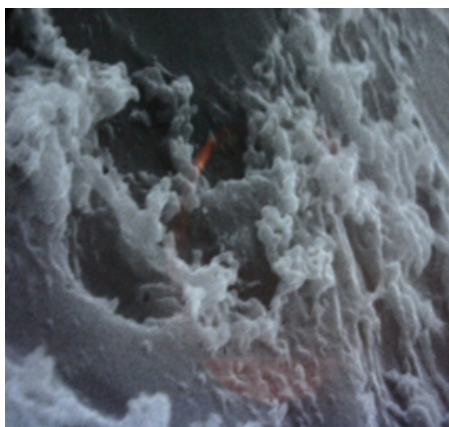
Figure 6. Morphology of the contact surface of removable dentures oral mucosa with "Ftorax" material. 400x magnification in SEM.
