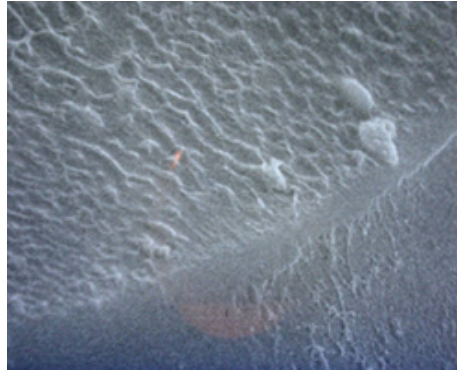
Figure 8. The relief of the prosthesis surface after bonding with "Gluma Comfort Bond" in SEM at a magnification of 200 times.
